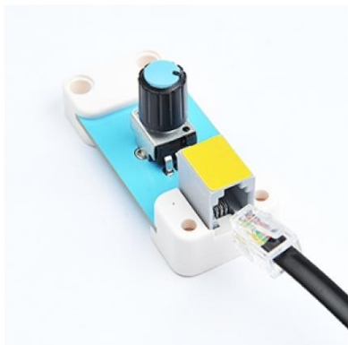
RJ11 wire(4P4C) is connected to the Planet X Sensor
